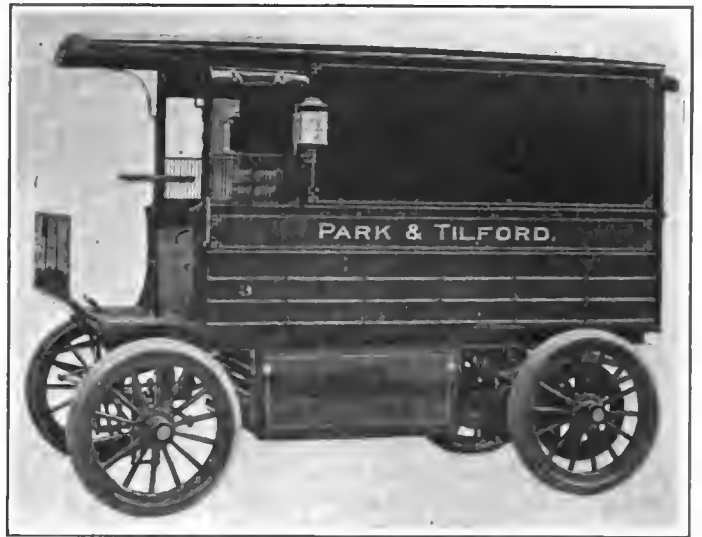
V. E. CO.'S TWO-TON ELECTRIC DELIVERY WAGON.
